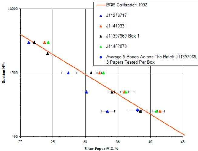
*Correlating New Batches of Whatman’s Filter Papers with the Original BRE Calibration.*
