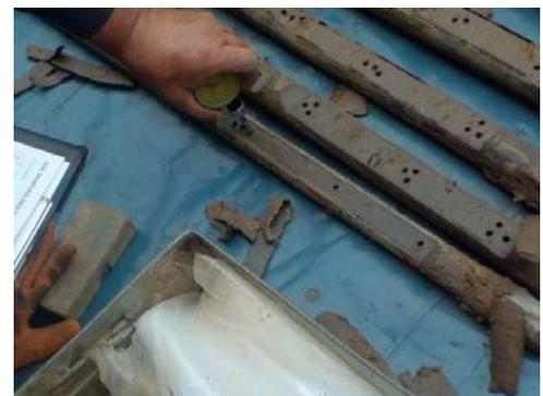
Left, oedometer and penetrometer tests reveal similar profiles. Above, readings are taken at 250mm ctrs from intact 'clumps' of clay soil using the penetrometer.
